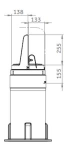
FUSE MOUNTING AREA MAXIMUM CAPACITY 6x FUSES
